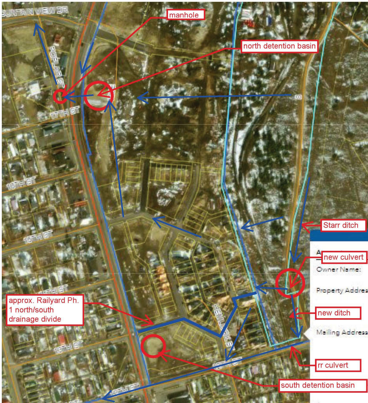
(Above: Lake County GIS map with staff notes on key existing or designed drainage features of Railyard development and surrounding area.)
