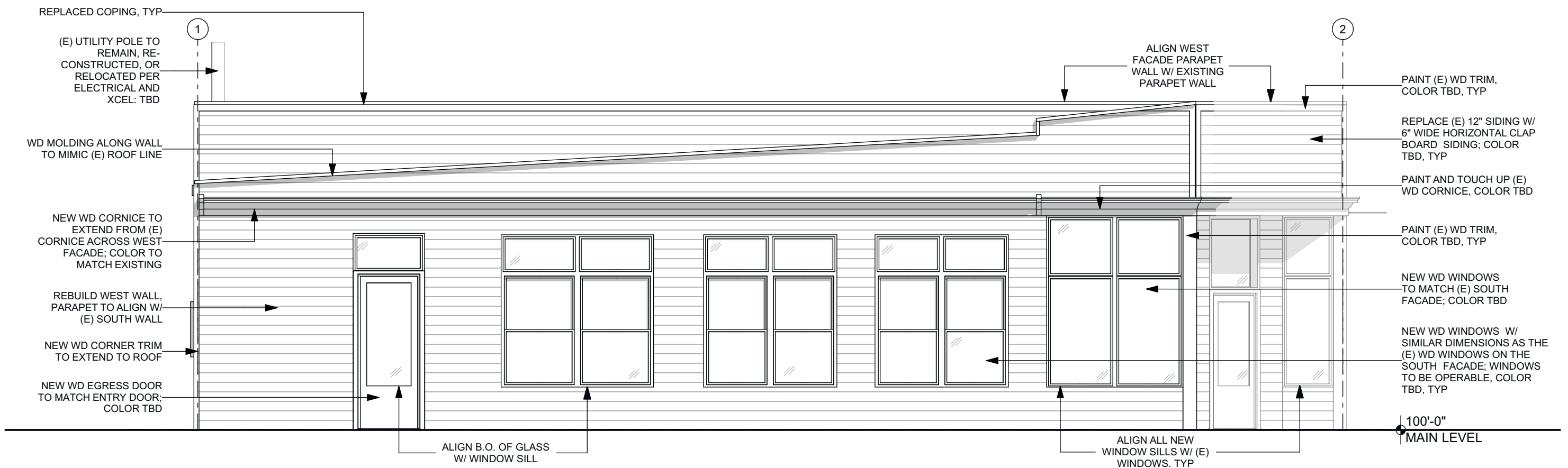
1 WEST ELEVATION: Parapet + Trim SCALE: 3/16" = 1'-0"
